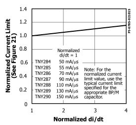
Figure 25. Standard Current Limit vs. di/dt.
