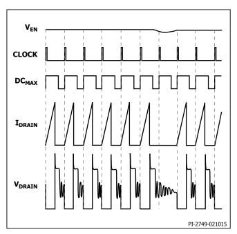
Figure 7. Operation at Near Maximum Loading.
