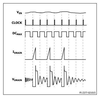
Figure 9. Operation at Medium Loading.
