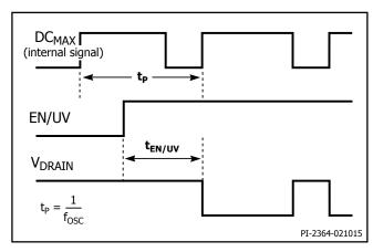
Figure 20. Output Enable Timing.
