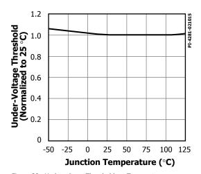
Figure 29. Undervoltage Threshold vs. Temperature.
