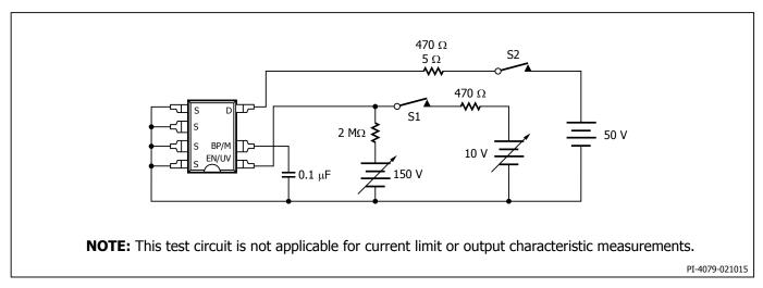
Figure 18. General Test Circuit.
