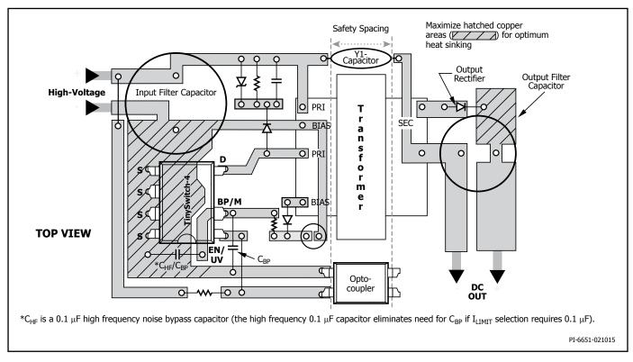
Figure 17. Recommended Circuit Board Layout for TinySwitch-4 with Undervoltage Lock Out Resistor.
