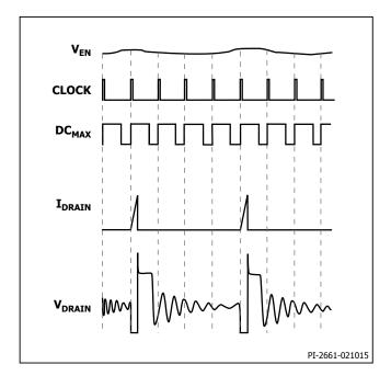
Figure 10. Operation at Very Light Load.
