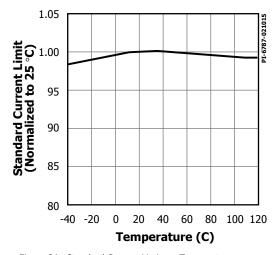
Figure 24. Standard Current Limit vs. Temperature.
