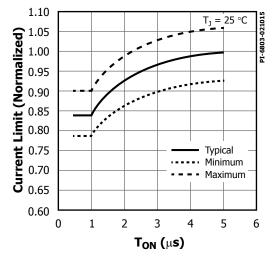
Figure 21. Current Limit vs.  $T_{\rm ON}$  for TNY284~287.
