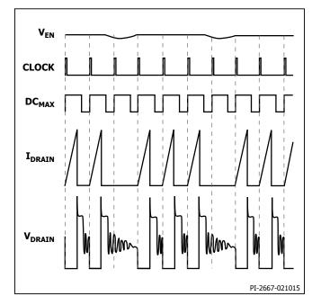
Figure 8. Operation at Moderately Heavy Loading.
