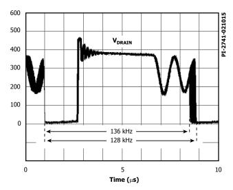
Figure 5. Frequency Jitter.
