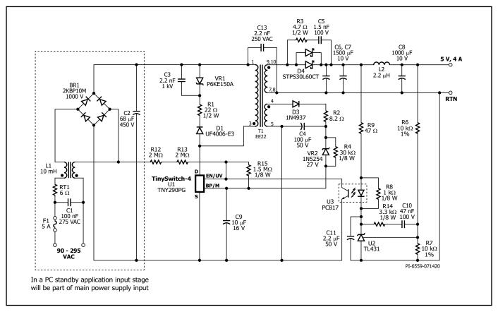
Figure 16. TNY290PG, 5 V, 4 A Universal Input Power Supply.
