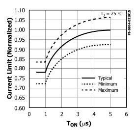
Figure 22. Current Limit vs.  $\rm T_{\rm ON}$  for TNY288~290.
