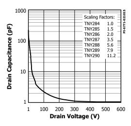
Figure 27.  $C_{OSS}$  vs. Drain Voltage.
