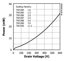
Figure 28. Drain Capacitance Power.
