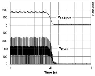
Figure 13. Normal Power-Down Timing (without UV).
