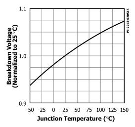
Figure 23. Breakdown vs. Temperature.
