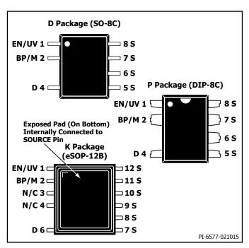
Figure 4. Pin Configuration.
