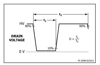
Figure 19. Duty Cycle Measurement.
